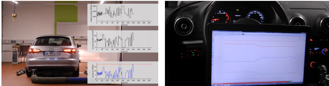
Figure 3: Dynamic safe Active Learning steering a car's engine to conduct measurements for a railpressure system. Experimental set-up connecting the car's engine to the Matlab based algorithm.
