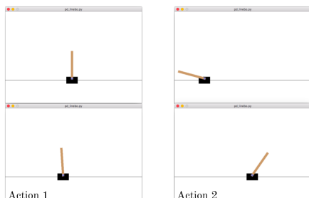
Figure 3: Cartpole setup. In each iteration, the subject indicates a preference between the cartpole behaviors resulting from different actions (controller parameters). Above, Action 1 (left) has higher reward than Action 2 (right).
